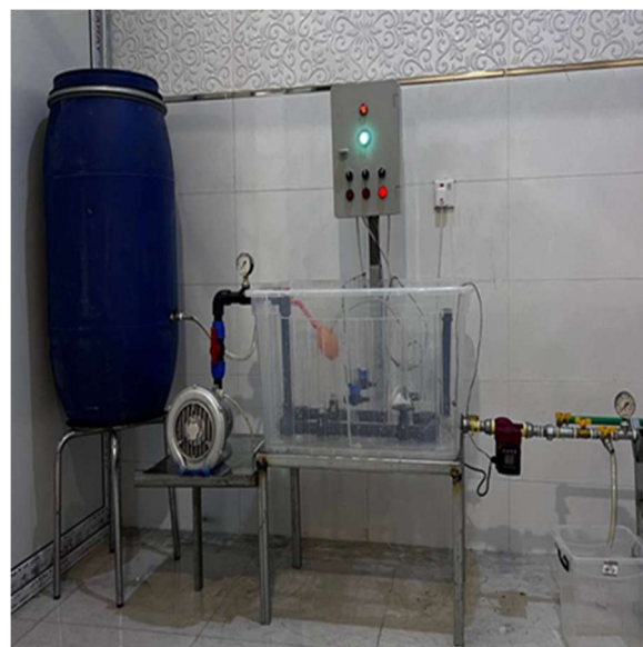
Figure 3. Sequencing Batch Biofilm Reactor (SBBR) Lab Scale Plant
