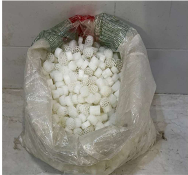
Figure 4. Bio Media Plastic carrier (moving bed biomedica)
